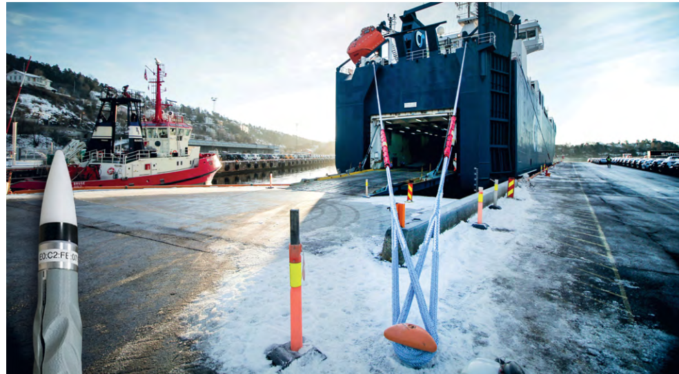
Bluetooth 5 tech's long range feature enables the smart rope to transmit wireless signals—in a tough environment dominated by RF absorbing substances such as steel and water—to a collector box sited up to 100 meters away from the sensor
